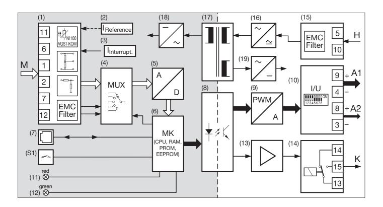
Fig. 3. Block diagram. In the case of the "intrinsically safe" version [EEx ia] IIC, the intrinsically safe circuits are those in the shaded area.
