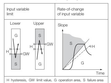
Fig. 6. Switching function according to limit monitored.
