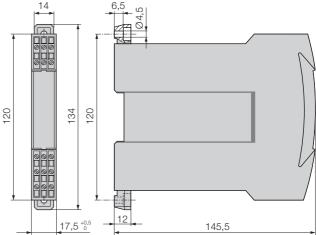
Fig. 7. SINEAX V 604 in housing **S17** clipped onto a top-hat rail  $(35 \times 15 \text{ mm} \text{ or } 35 \times 7.5 \text{ mm}, \text{ acc. to EN 50 022}).$
